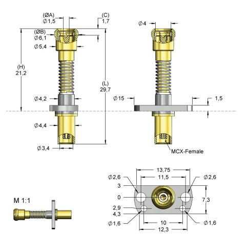
The flange mounting in combination with the wobble function of the probe enables safe contacting in the smallest possible center for Fakra connectors. Cable connection with standard connector MCX-male.
