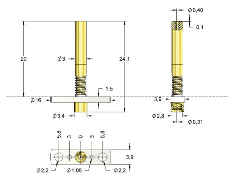
The probe can be mounted using the flange. Cable connection with standard connector Mini SMP female.
