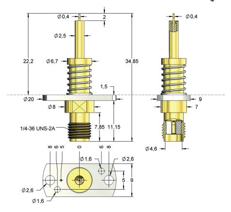
The probe can be mounted using the flange. Cable connection with standard connector SMA male.
