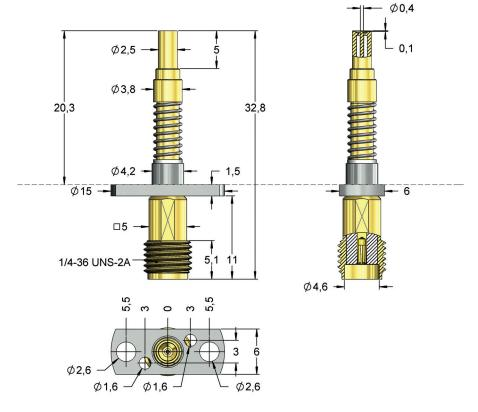
The probe can be mounted using the flange. Cable connection with standard connector SMA male.
