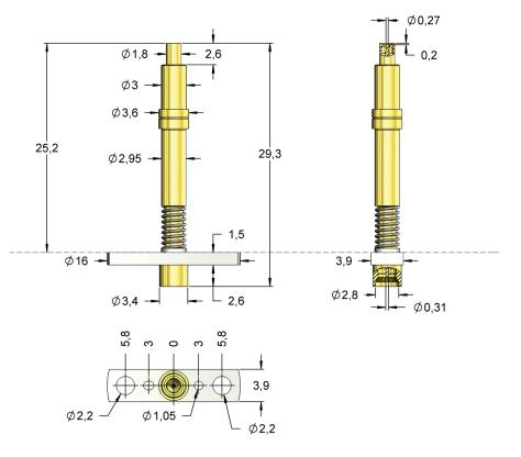
The probe can be mounted using the flange. Cable connection with standard connector Mini SMP female.
