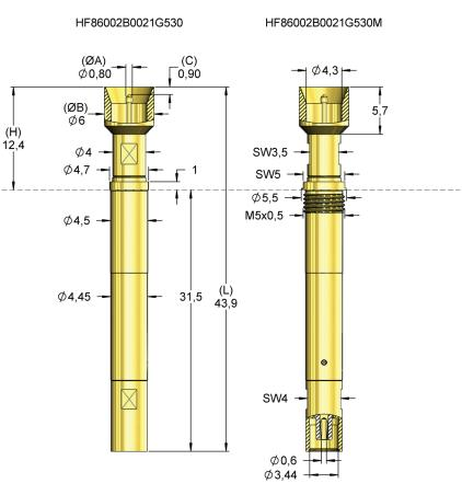
For contacting DIN 1,0/2,3-Female connectors.
