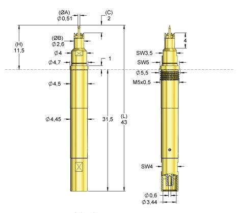
For contacting PCBs coaxial closed.
