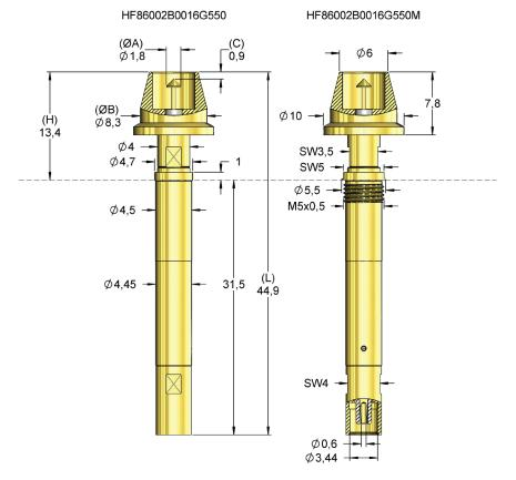
For contacting BNC-Female connectors.
