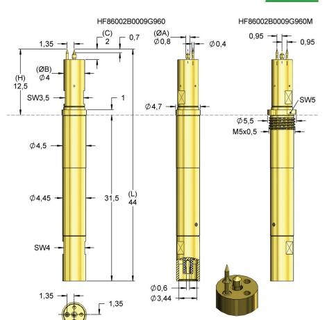
For contacting PCBs. The signal pin is not spring loaded. The ground pins have a spring force of 80 cN. Suitable mounting receptacles see H860 or H860FL.
