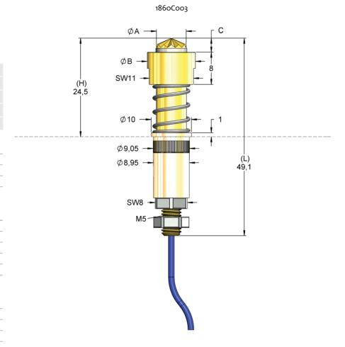
The M5 thread can be mounted with a counternut to a cable eye.
